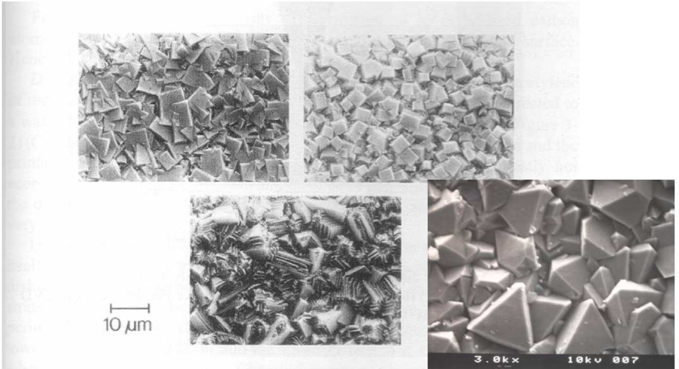
Figure 3-20. Diamond films (on a SIALON surface) deposited by microwave activation of 1.7 % methane in hydrogen. The different morphologies originate from different gas pressures and different microwave powers.
